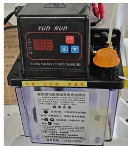
Auto Lubrication Tank
