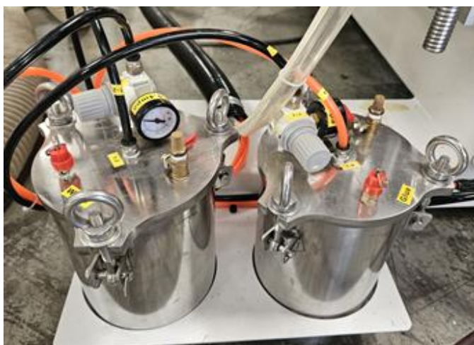
Glue & Cleaning Water Tank
